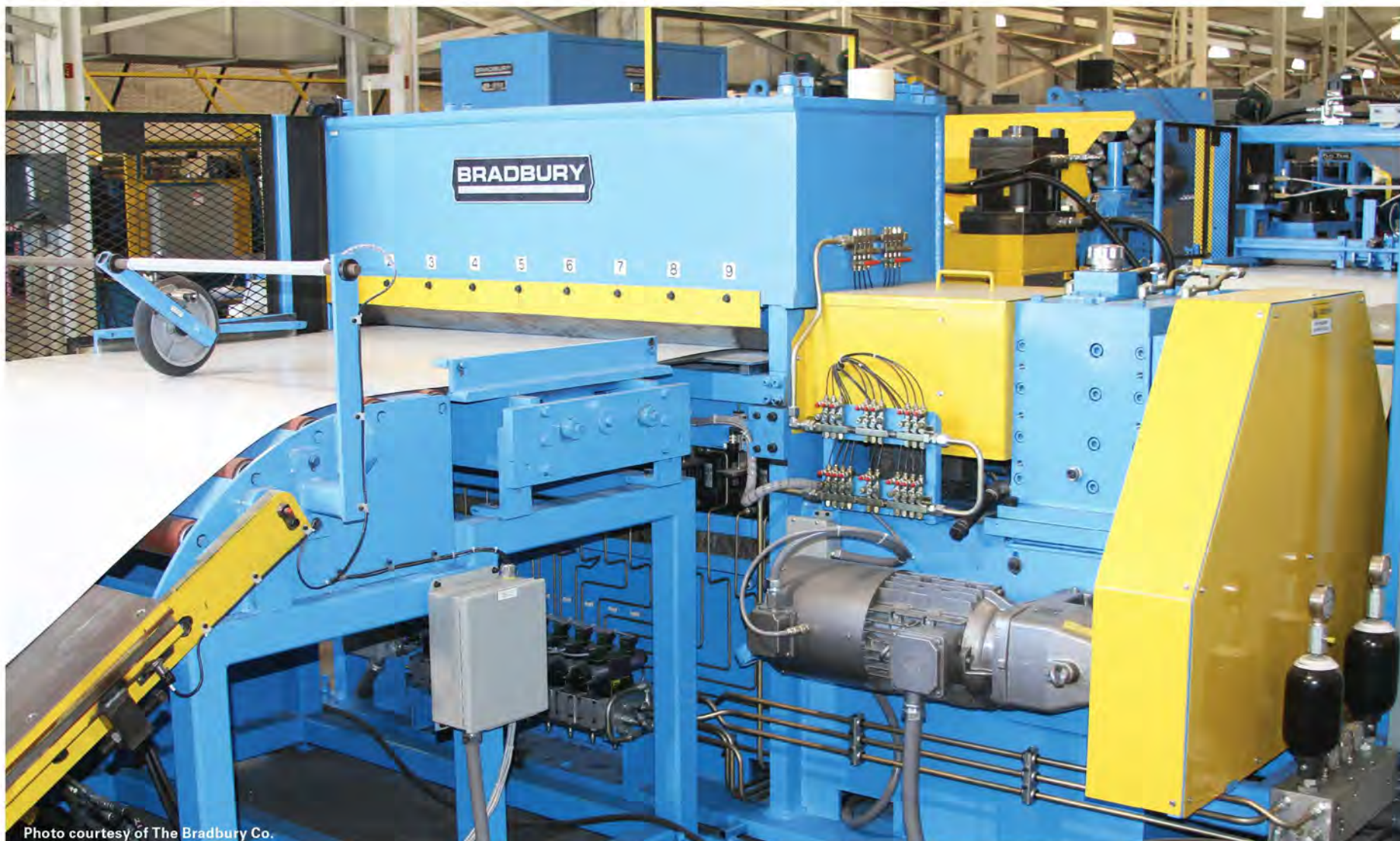
This is a Hydraulic Leveler, similar to a model that would be used to spec a standing seam or architectural panel line.
