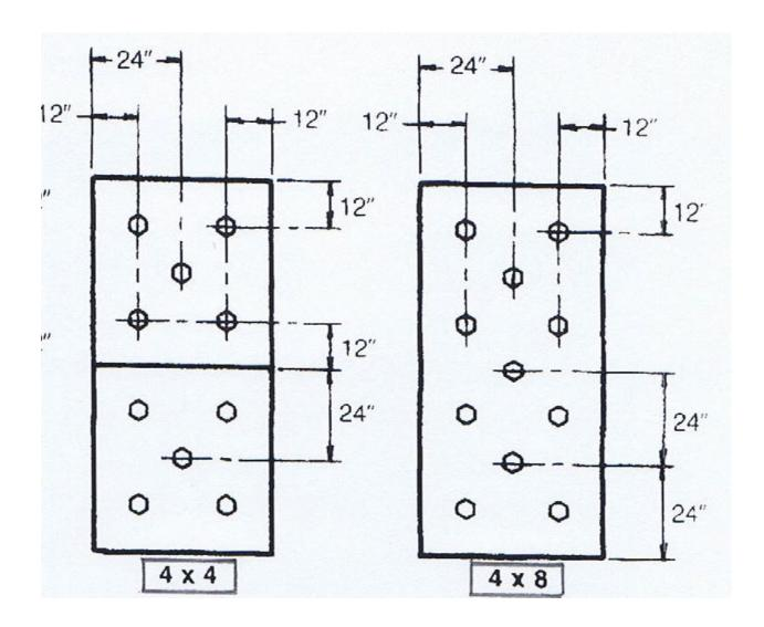
Figure 1. Insulation Fastening Patterns
