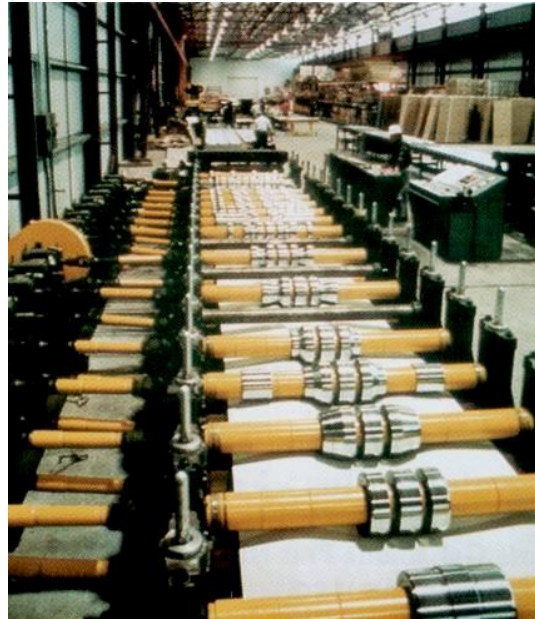
ACRYLUME ® Sheet can be roll-formed without use of oil
