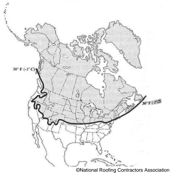
Figure 10-24 Example of North America Temperature Chart January Temperatures 30° F or Less
