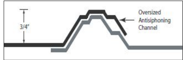
Figure 5-7 Typical Trapezoidal Rib with Overlap Seam
