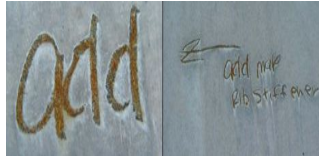
Figure 10-45 Corrosion Caused by Graphite Pencil
