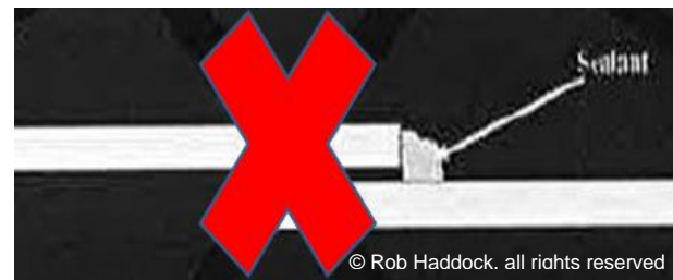
Figure 15-15 Butyl Sealant Should NOT be Externally Applied
